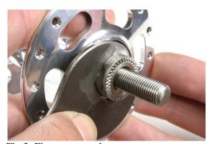
Fig.3 Fit cone wrench onto cone nut.
