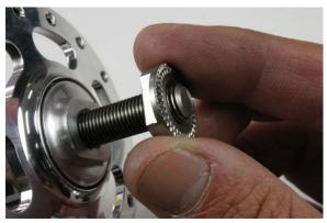
Fig.15 Installing steel lock nut.
