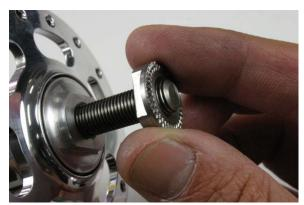
Fig.5 Remove lock nut.
