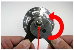
Fig.4 Turn steel lock nut counter-clockwise.
