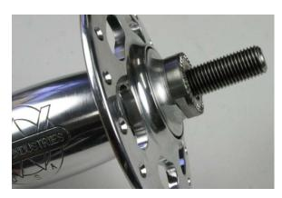
Fig.13 Axle is fully seated.
