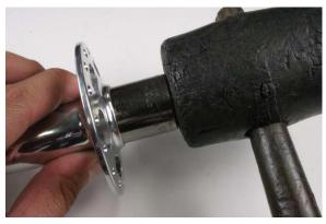
Fig.10 Fully seat bearing in bore.
