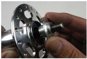
Fig.6 Remove cone nut.
