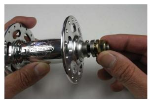
Fig.1. Removing axle nuts.
