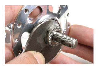
Fig.16 Wrench on flats of cone nut.
