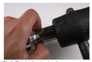
Fig.9 Tapping bearing into bore.
