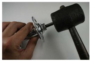
Fig.12 Tap axle end to fully seat.
