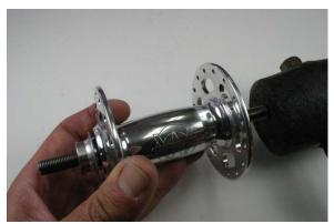
Fig.7 Tap axle assembly out of shell.
