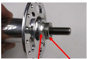
Fig.2 Aluminum.cone nut. Steel lock nut.
