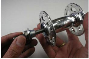
Fig.8 Withdraw axle assembly from shell.
