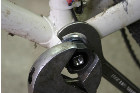
Fig.9 Hold cup while lock ring is tightened.
