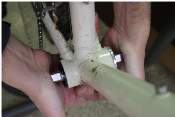
Fig.10 Checking for lateral play.
