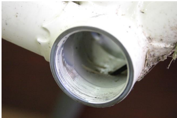
Fig.1 BB threads clean and ready for install.
