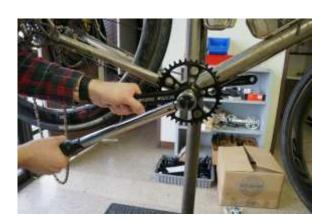
Fig.8 Torque to 50 Nm.
