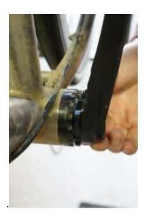
Fig.9 Adjustment ring placement.
