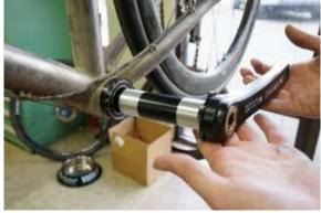
Fig.6 Installing spindle w/ arm in place.
