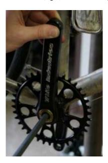
Fig.7 Crank arms clocked 180 degrees
