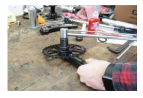
Fig.4 Tighten locking ring
