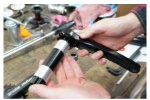
Fig.5 Mating spindle to arm
