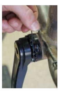
Fig.10 Cinch down adjustment ring
