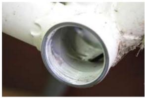
Fig.1 BB threads clean and ready for install.
