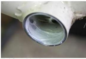
Fig.2 Greased threads.
